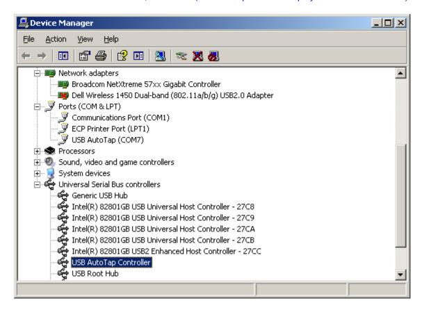
\*\*\*For AutoTap Diagnostic (V3.1 or V2.05 software), your AutoTap must be assigned between com 1 and 16. I highly recommend avoiding com 3.
