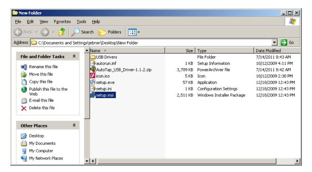
After the drivers have completed the installation process, connect the AutoTap hardware to a USB port and then go into Device Manager to confirm that the AutoTap is listed under both the Universal Serial Bus Controllers, and Ports. (Some computers will display this as Other Devices)
