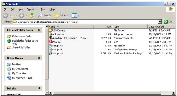
Make sure your AutoTap hardware unit is NOT connected to your computer USB port, then double click on the setup.msi file. **The drivers will show up as Ulinx USB drivers during installation.** For Windows Vista and Windows 7, you will need to click on the blue and yellow shield that appears in the task bar, then click on Allow. You may need to click on Allow more than once for Windows 7 to complete the driver installation.
